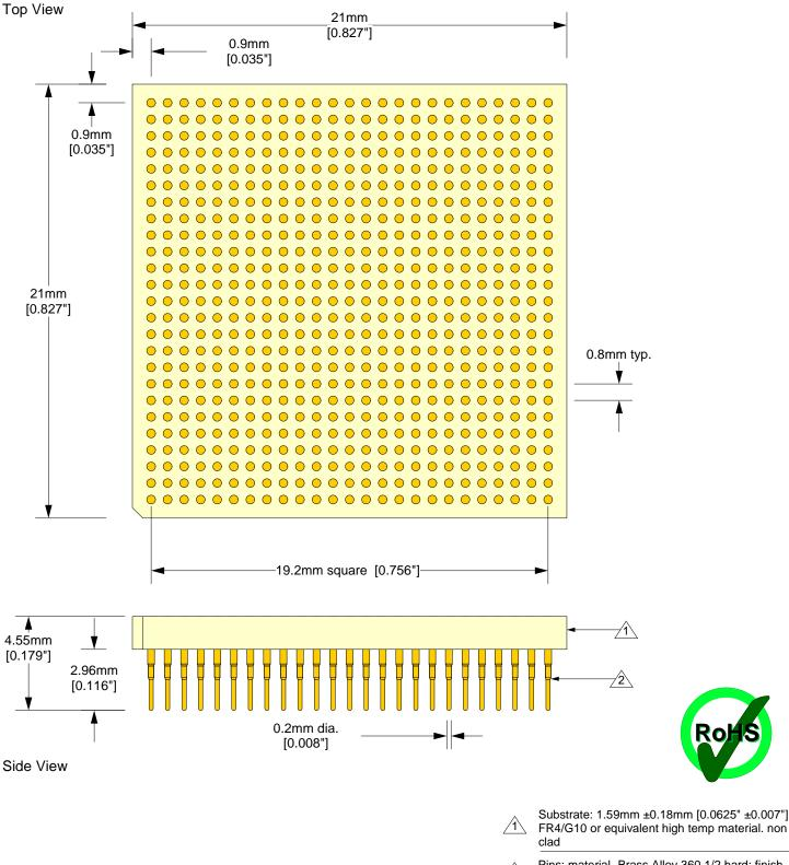
Pins: material- Brass Alloy 360 1/2 hard; finish-0.25µm [10µ"] Au over 1.27µm [50µ"] Ni (min.).
